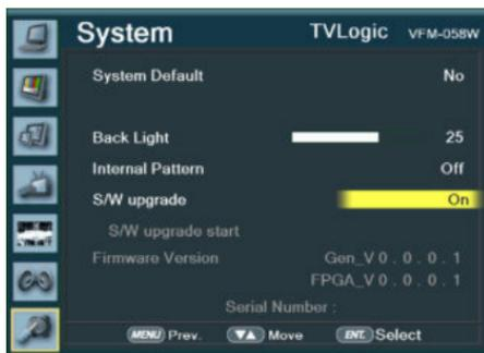
• USB memory stick(Thumb drive) that has F/W is necessary.
