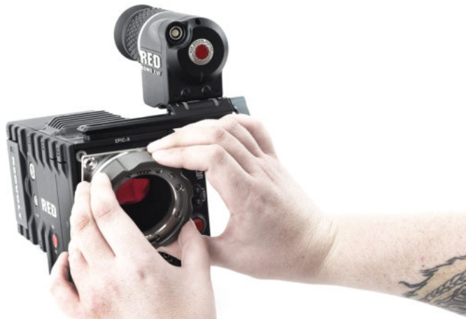
Figure: Remove the Lens Mount
