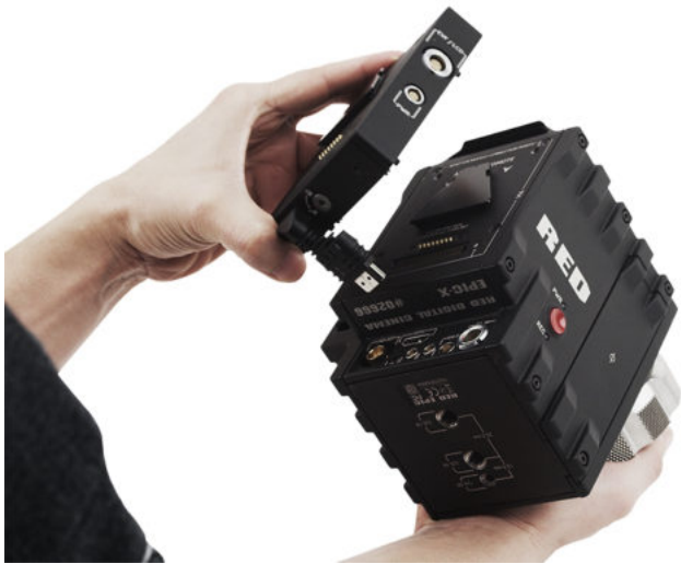
Figure: Install +1 Adaptor Module
