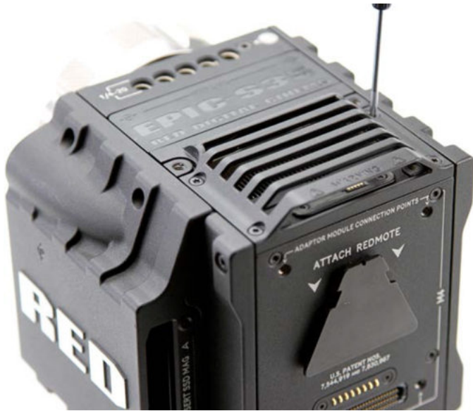
Figure: Replace the Hood Scoop
