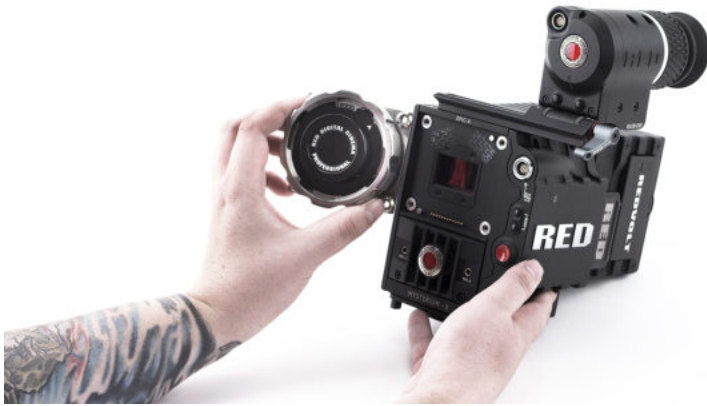
Figure: Align Lens Mount Pins
