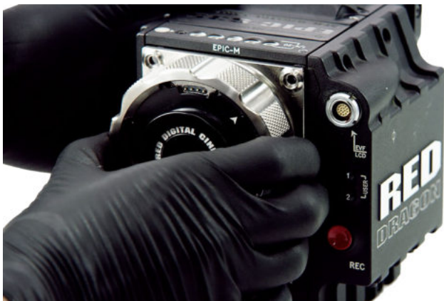
Figure: Remove Lens Mount
