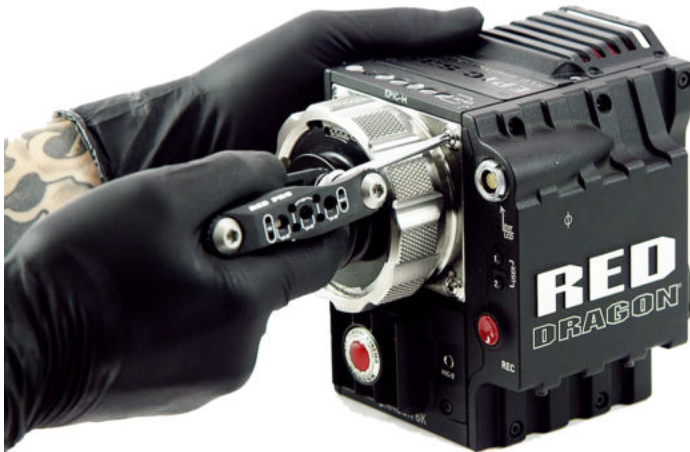
Figure: Replace Lens Mount
