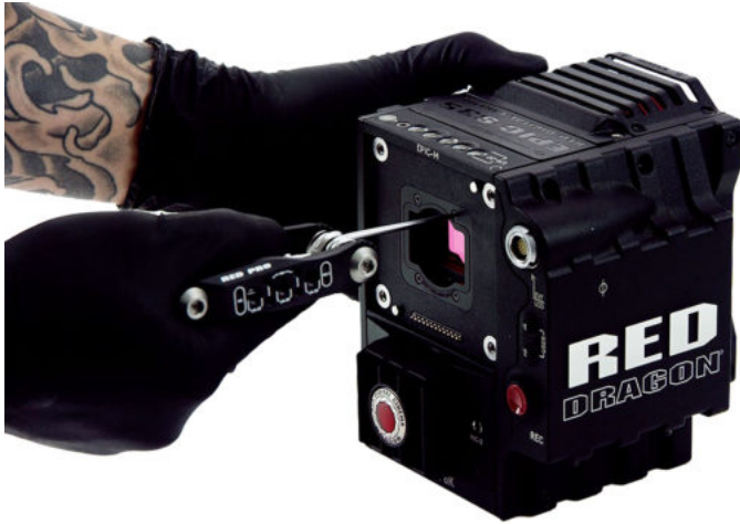
Figure: Remove OLPF Module Screws
