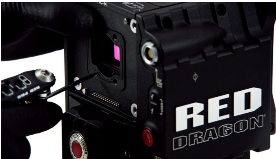
Figure: Replace the OLPF Module and Screws
