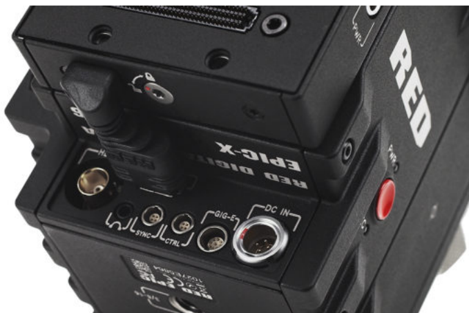
Figure: Insert HDMI Connector into the BRAIN
