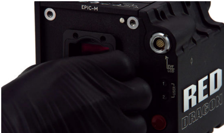
Figure: Remove the OLPF Module
