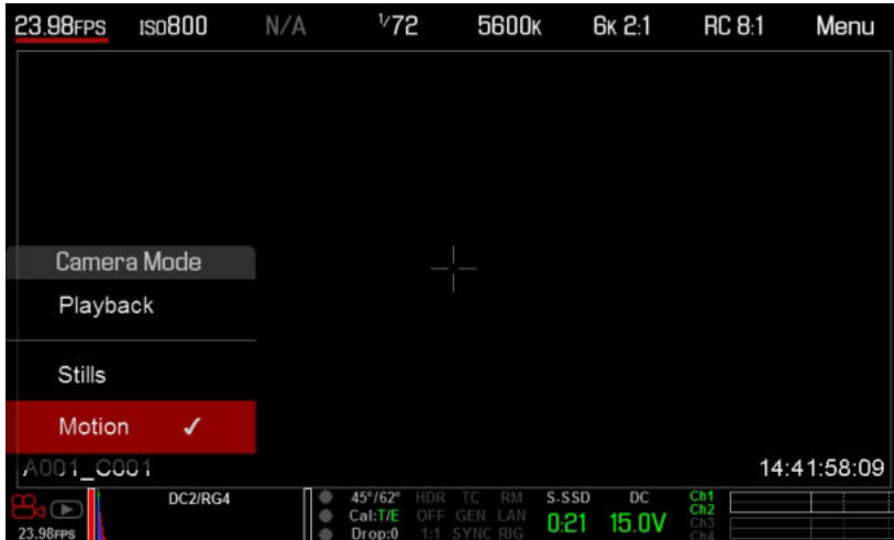
Figure: Swipe Up to Select a Camera Mode
