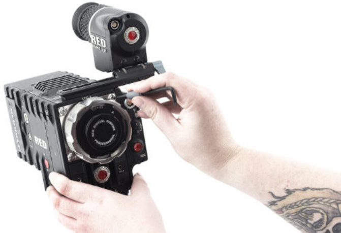
Figure: Remove the Lens Mount Screws
