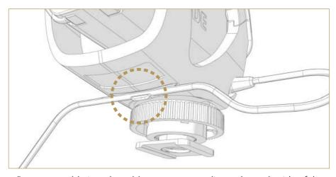
Press your cable into the cable management clip on the underside of the shock mount cradle
