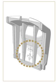
Insert the battery with the negative terminal on top
