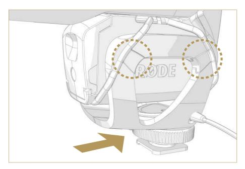
Slide the tapered square on the middle of the band into the notch on the shock mount. Note the orientation of the cradle has the shoe mount closer to the rear of the microphone
