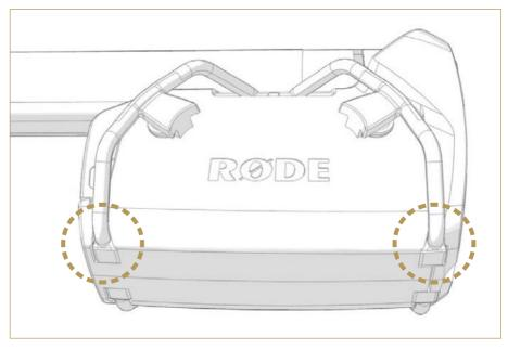
Angle the square end of the band into the corresponding square notch on the underside of the mic body
