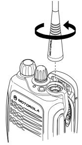
1. Turn the antenna counterclockwise until you can remove it.
