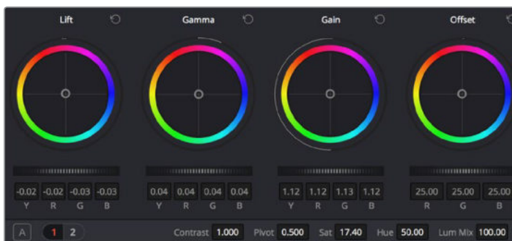
The 'lift', 'gamma', 'gain' and 'offset' color wheels give you total control over the color and tonal balance of your clips. To make a uniform adjustment to all colors for each tonal region, drag the dial underneath the color wheels back and forth.
