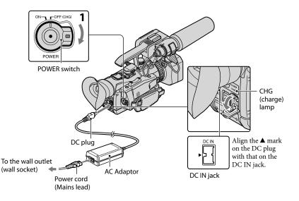
You can charge the "InfoLITHIUM" battery pack (V series) after attaching it to your camcorder.
