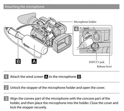
Be sure to place the microphone with the model name (ECM-XM1) facing upward.
