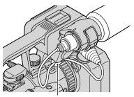
Hook the cable in the outer cable holder.
