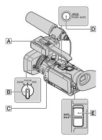
You can adjust the iris, gain, shutter speed or white balance manually.
