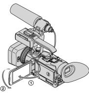
Open the LCD panel 90 degrees to the camcorder (①), then rotate it 180 degrees to the lens side (②).
