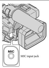
When an external microphone is connected to the MIC input jack, sound is switched to that of the external microphone. Sound is not switched during recording.
