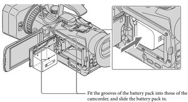
Close the LCD screen of the camcorder (③) after closing the battery cover (①②).
