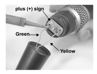
**NOTE:** On older models, there may be a third, black wire. Connect this wire to the case ground nut between the green and yellow terminals on the cartridge.
