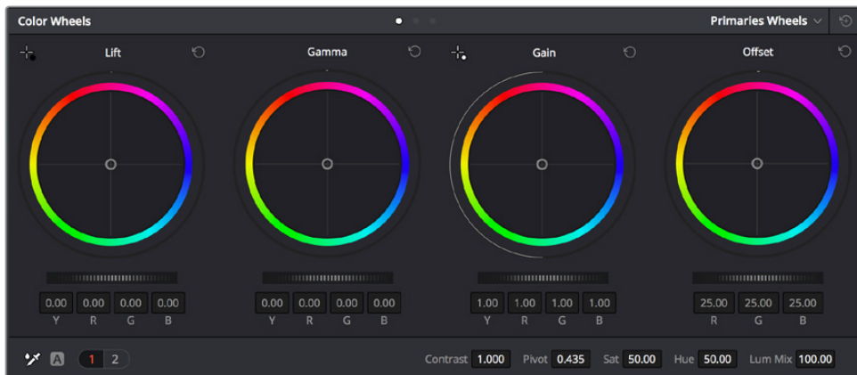
The 'lift', 'gamma', 'gain' and 'offset' color wheels give you total control over the color and tonal balance of your clips. To make a uniform adjustment to all colors for each tonal region, drag the dial underneath the color wheels back and forth
