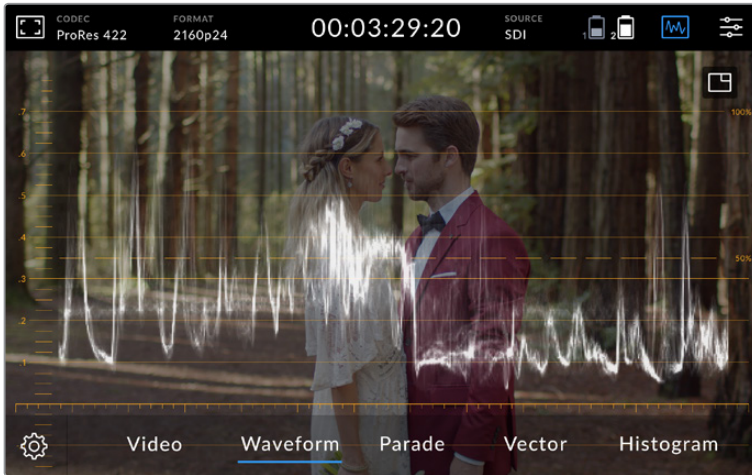
The waveform display showing luminance values
