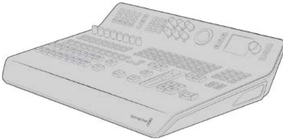
ATEM Television Studio Pro models has a console style control panel similar to an ATEM advanced panel
