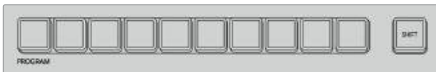
Press any of the source buttons on the program row to perform a cut transition from the program bus
