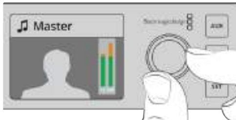
Use the knob to adjust the master audio level and you can see the effect on the main audio meters in the LCD
