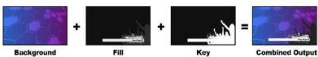
Combining a background, fill and key in a linear key
