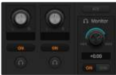
The monitor volume knob and sliders set the independent audio levels for monitoring the program audio together with talkback and sidetone, plus the overall volume of the mix.
