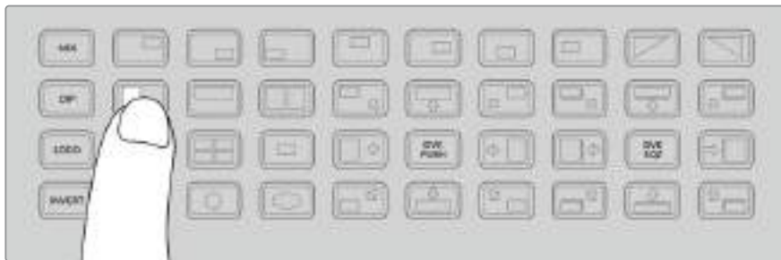
The transition pattern buttons let you choose which pattern to use in a transition, such as a horizontal wipe
