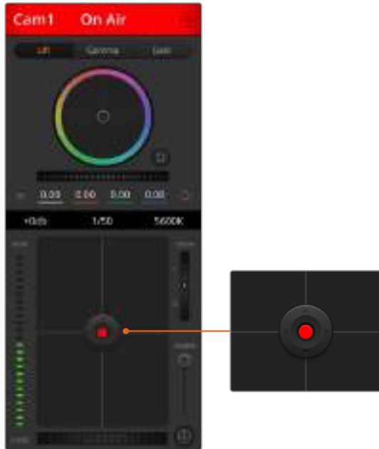
The iris/pedestal control illuminates red when its respective camera is on air.
