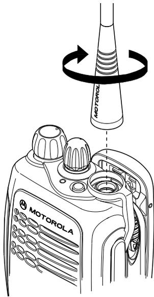
1. Align the threaded end of the antenna with the radio's antenna connector.
