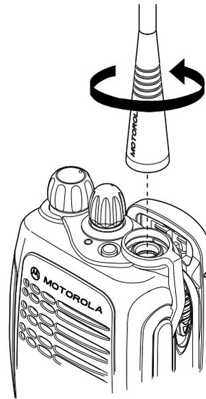
1. Turn the antenna counterclockwise until you can remove it.
