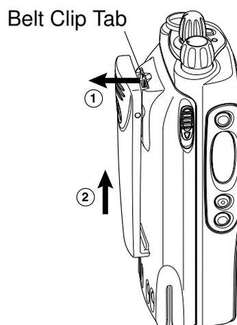
1. Use a key to press the belt clip tab away from the battery.
