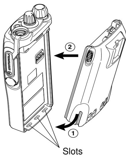
1. Fit the extensions at the bottom of the battery into the slots at the bottom of the radio's body.
