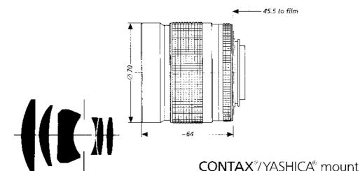
The 85 mm Planar® T\* f/1.4 lens ranks amongst the best high-speed lenses presently available for 35 mm reflex cameras. An outstanding feature is the excellent image quality even at full aperture. This feature results in special applications of the 85 mm **Planar**® T\* f/1.4 lens for discerning amateur and professional photographers. Owing to the fully utilizable speed, this lens is especially suitable for stage photography. Sporting events, outdoors and
