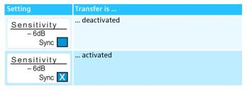
Via the "Sync" menu item, you can transfer the parameters from the receiver to the transmitters via the infra-red interface (see page 19).
