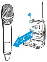
The parameters are transferred to the transmitter. When the transfer is completed, " $\checkmark$ " appears on the display panel of the diversity receiver. The receiver then switches back to the current standard display.
