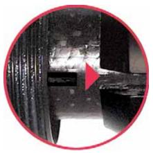
If a user opens the hand nut more than 5 turns then the pin can come out of its location in the ring. Then when the screwlock is retightenend the pin may move away from its slot and will be bent or broken by the compression ring, which will be also be scored.
