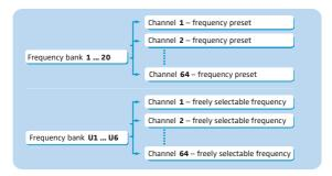
Each of the channels in the frequency banks "1" to "20" has been factory-preset to a fixed frequency (frequency preset). The factory-preset frequencies within one frequency bank are intermodulation-free. These frequencies cannot be changed.
