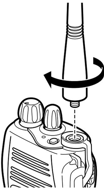
1. Align the threaded end of the antenna with the radio's antenna connector.
