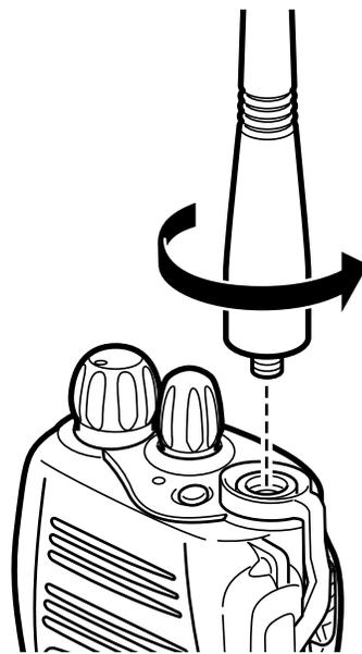
1. Turn the antenna counterclockwise until you can remove it.
