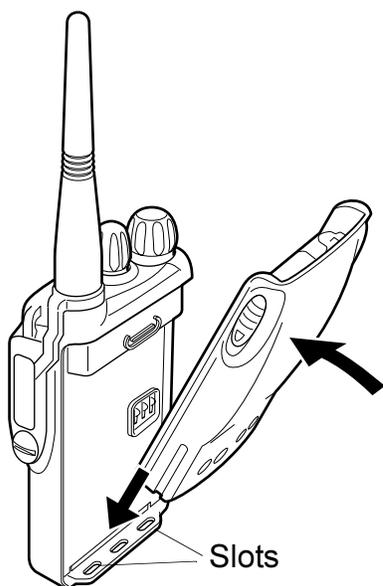
1. Fit the extensions at the bottom of the battery into the slots at the bottom of the radio's body.
