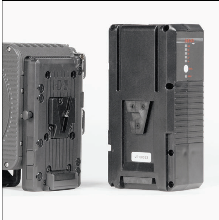
Figure 14: ALEXA with BAB-V and V-Mount battery
