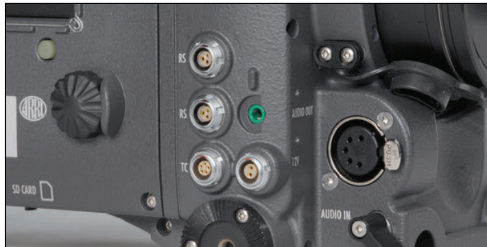
Figure 16: 24 V outputs (RS) and 12 V output
