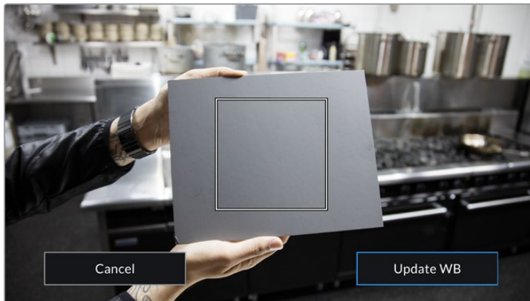
Tapping the 'AWB' icon in the white balance menu will bring up the auto white balance screen. Use this with a white or neutral grey surface to automatically set a neutral white balance
