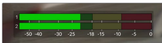
The colored bars on the audio meter represent peak audio levels. Ideally your peak audio levels should fall in the upper end of the green zone. If your peaks enter into the yellow or red zones your audio is in danger of clipping.
