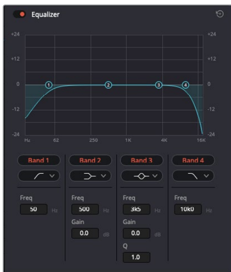
The four band equalizer can be applied to every clip in the timeline
