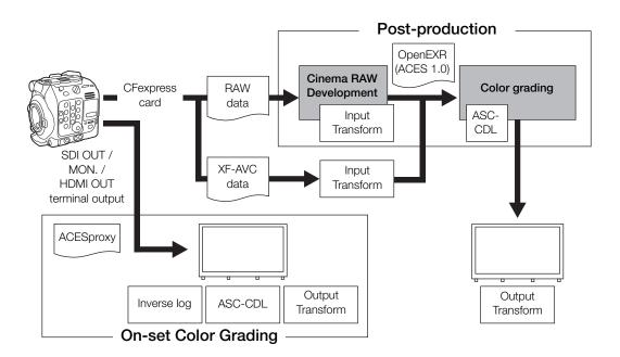
ACESproxy: ACESproxy video data that is output from the camera's output terminals when performing
