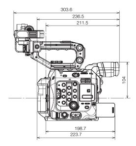
Camera with camera grip, handle unit, microphone holder, LCD monitor (open), LCD attachment unit and optional EU-V2 Expansion Unit 2
