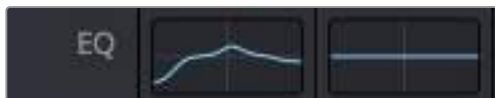
The EQ section in the mixer panel indicating an EQ curve has been applied to track one
