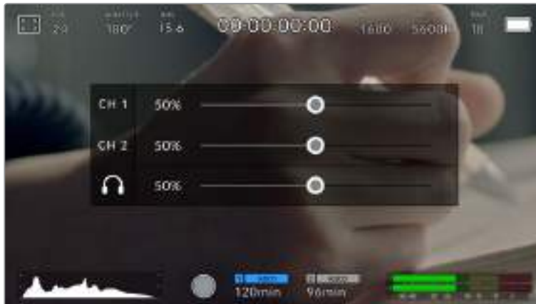
Tap the audio meters on the LCD touchscreen to easily access volume and headset or speaker settings
