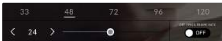
Tap the arrows on either side of the project frame rate or move the slider to make adjustments
