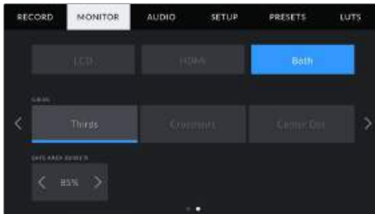
Page 2 of 'monitor' options for both LCD and HDMI on Pocket Cinema Camera 4K
