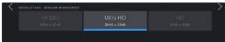
Pocket Cinema Camera 4K 'resolution' options. Note that in 4K DCI format the category is 'resolution', otherwise it's 'resolution - sensor windowed'.
