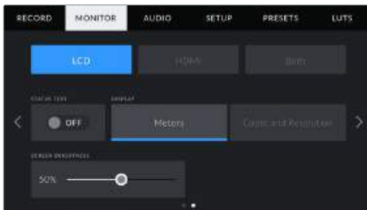
'Status text' gives you a clear view of your camera's preview image
