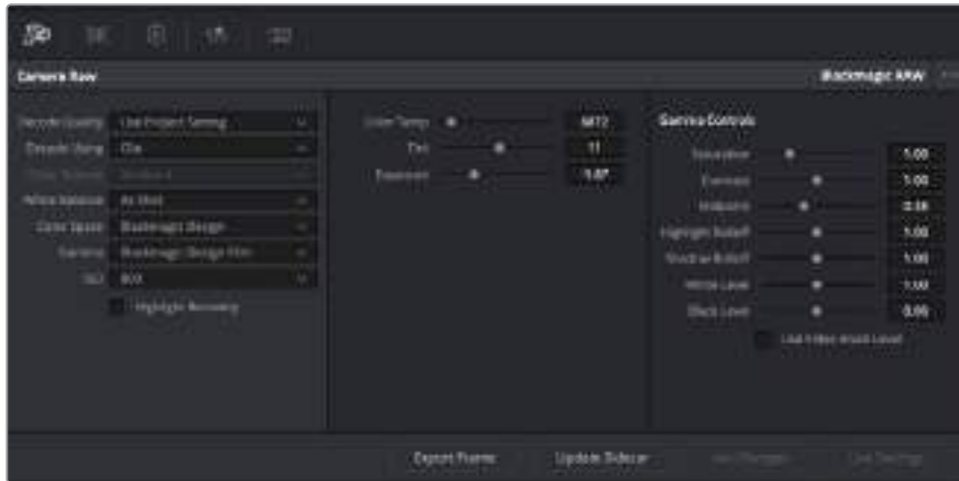
In the 'camera raw' tab, select 'clip' from the 'decode using' drop down menu to make adjustments to your clip's Blackmagic RAW settings
