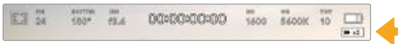
The shuttle speed indicator displays the speed and direction of footage being fast forwarded or reversed
